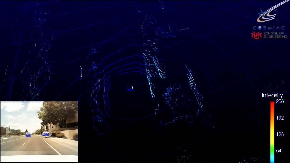
Mask—RCNN on Intel E3—1535m v5 CPU, Inference time for a frame : 3341 ms
